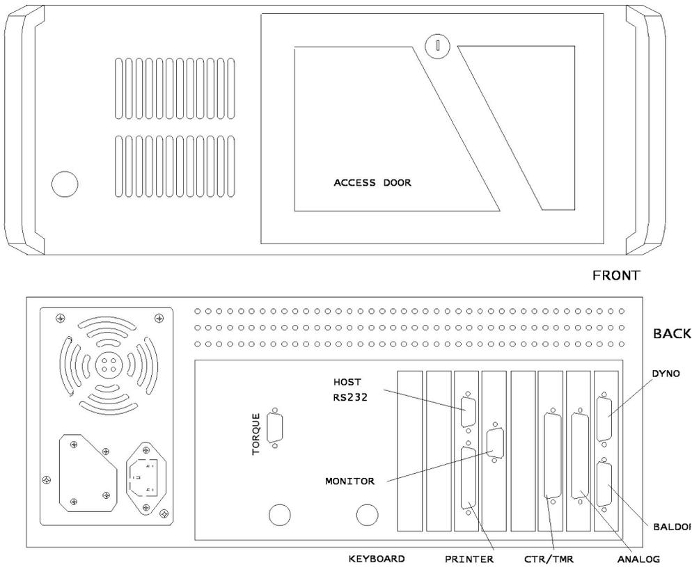
Figure 5. Front and rear views of the standard ARTIC-2 Dynamometer Controller. The Controller can be either desk-top or rack-mount configuration.
