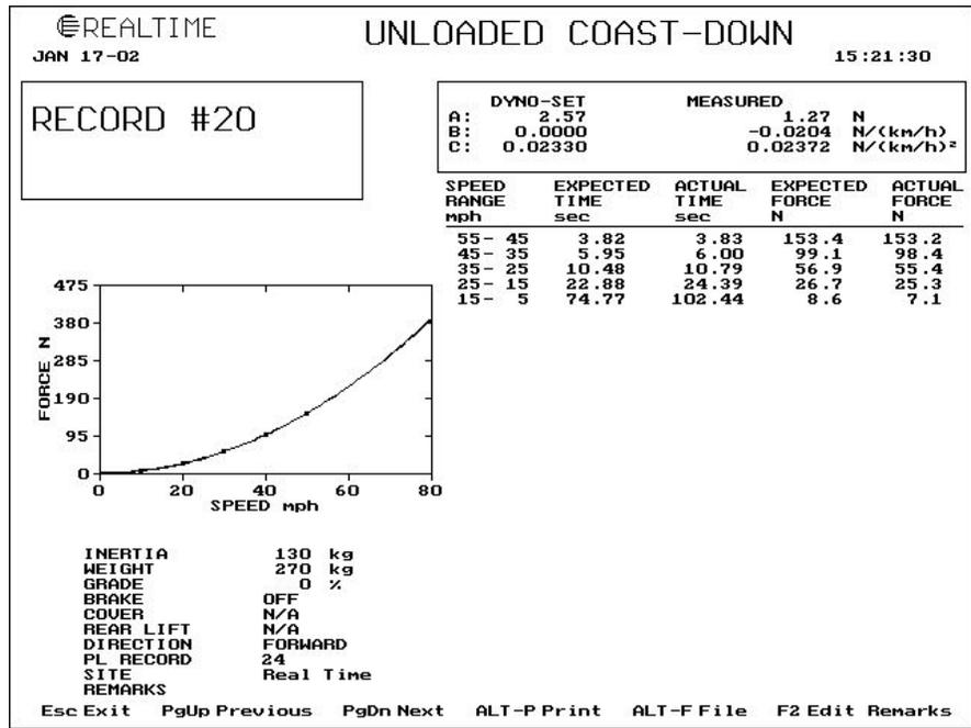
**Figure 2. The Unloaded Coast-Down screen from a motorcycle dynamometer.**
