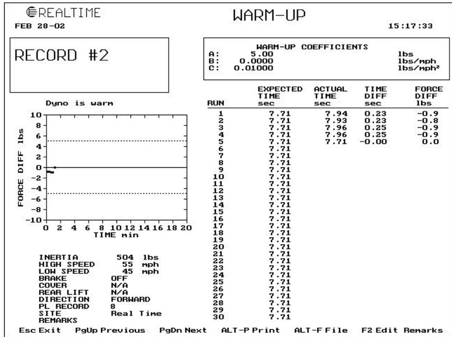
Figure 4. The Warm-up record from a motorcycle dynamometer.
