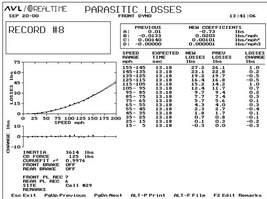
**Figure 3. The Parasitic Loss calibration screen from a mileage accumulation 4WD dynamometer.**
